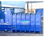
Compactor HL5 or HL20 containers: These containers are designed to attach to compactor machines, allowing optimum wastepaper payloads and are ideal for loose cardboard, printers waste, production spoils, converting operations or any other large volume, wastepaper generators - Sizes available from 25 to 50 yard<sup>3</sup> available.
