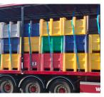
Cages / stillages / tubs: These collection systems are ideal for areas that have volumes of waste spread across wide areas, or ideal for internal storage of waste before being brought to a central point and are easily moved by forklift or pallet truck. Typical capacity per tub is 500 litres or up to 150kg of wastepaper (dependant on nature and type of papers)
